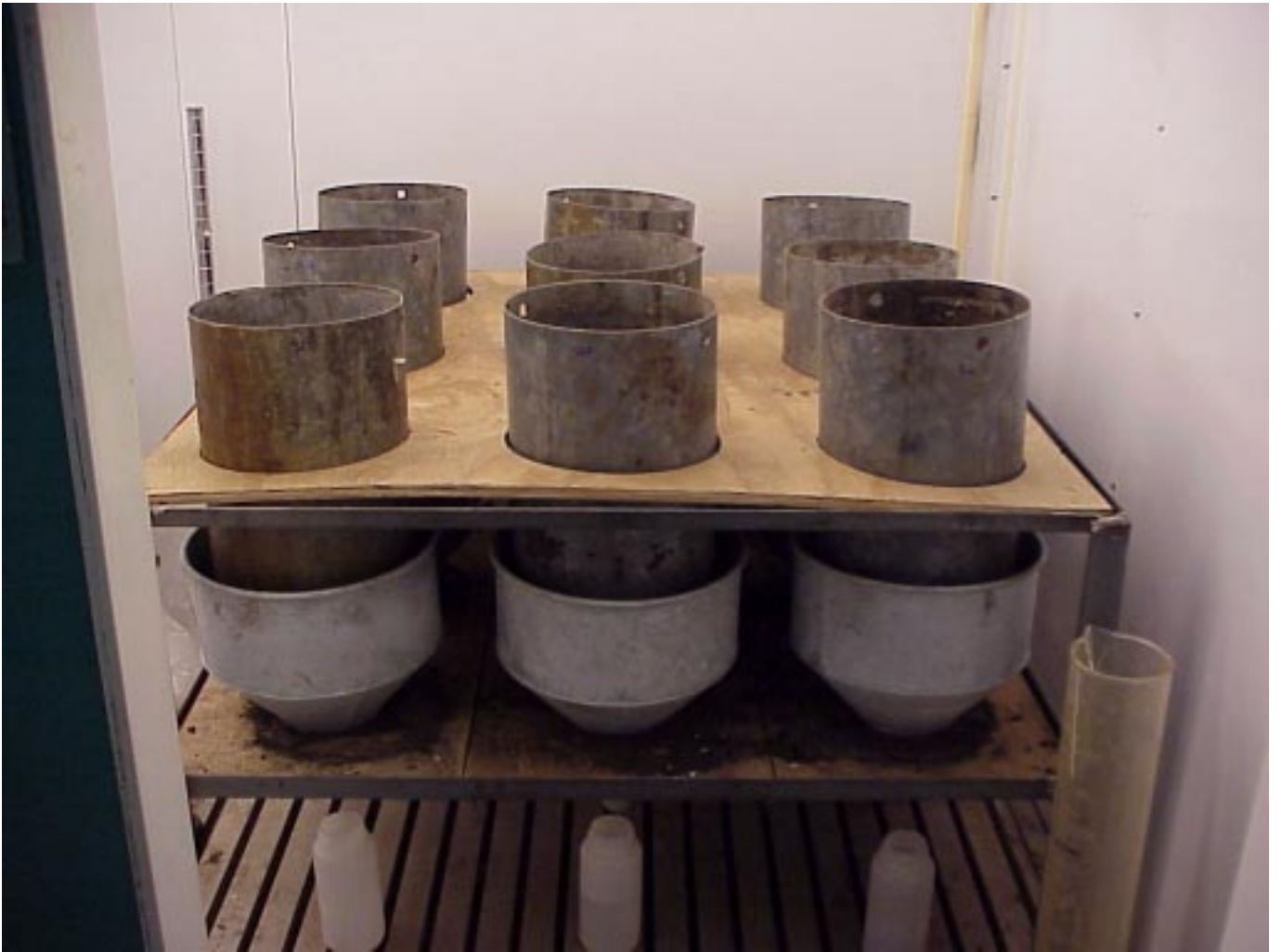
Figure 14. Spring soil columns in the leachate collection apparatus.
