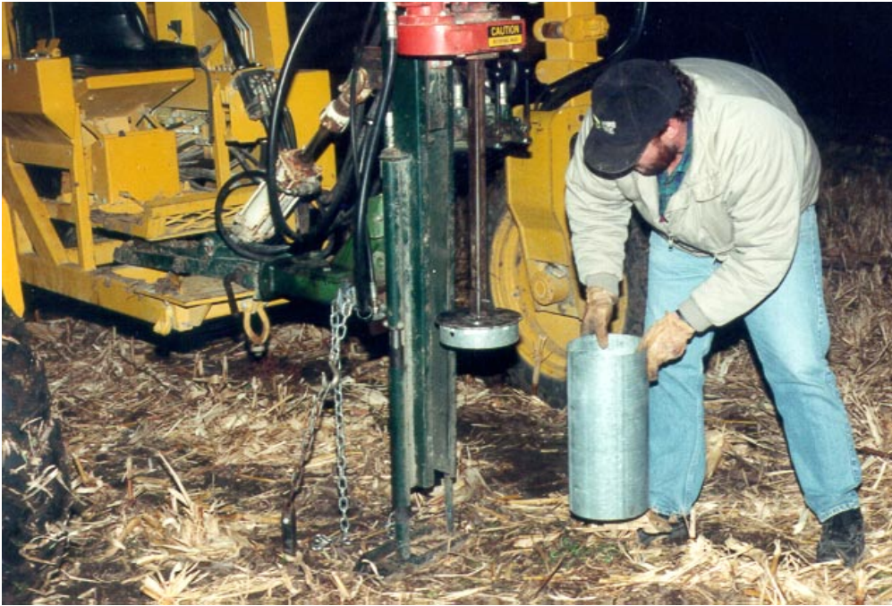
Figure 12. Positioning tubing for soil column extraction with the Giddings probe.
