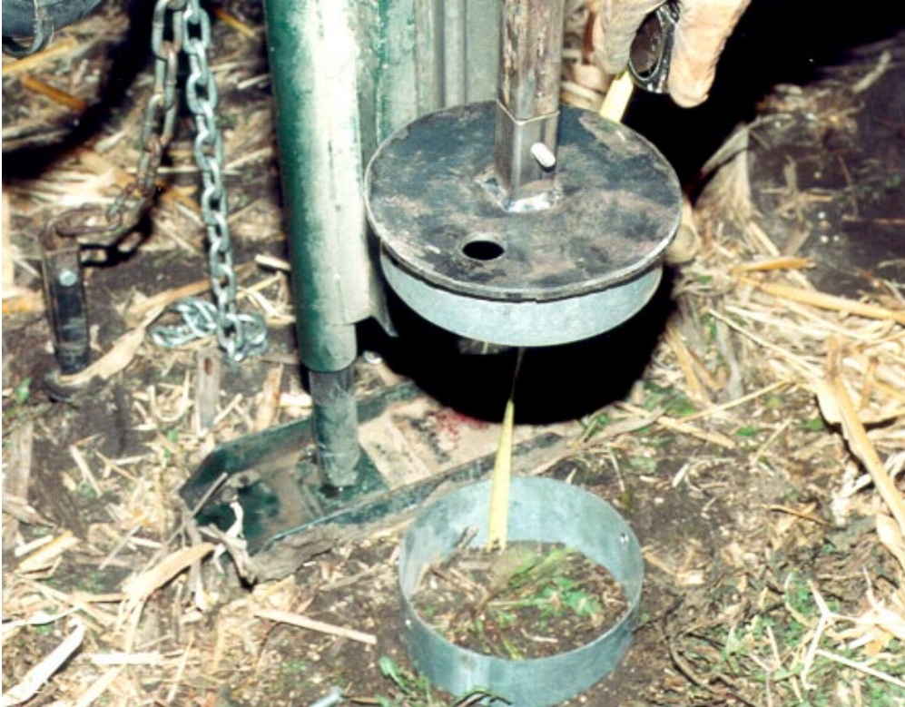
Figure 13. Measuring the soil column for compaction.
